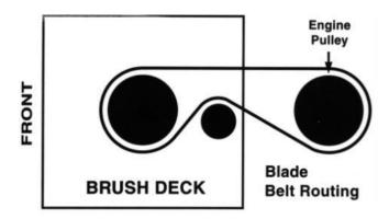
This label shows the proper routing of the drive belt. (#164371)
